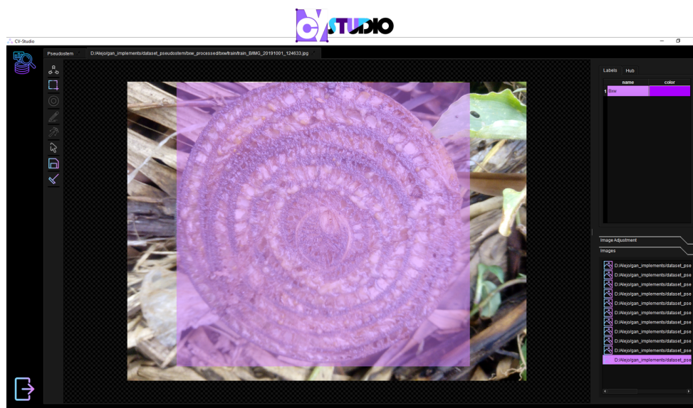
Figure 9.6: CVstudio software overview and labeling process, purple rectangle is an example of a bounding box which is the region of interest for the model.
