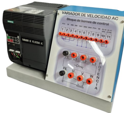
Figure 42. Siemens Micromaster 6SE9 221-8CC13 Variable Frequency Drive.
