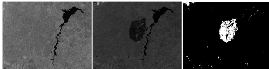
Figure 3.3: Omodeo. From left to right to the pre-event image, the post-event image and the change map (groundtruth)
