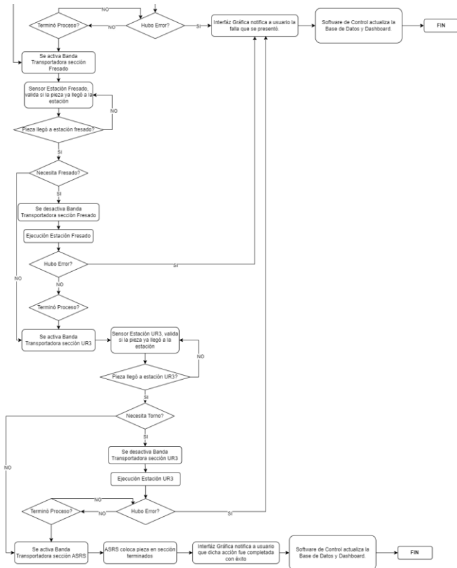
Figure 15: Control Software Functional Logic Part 2
