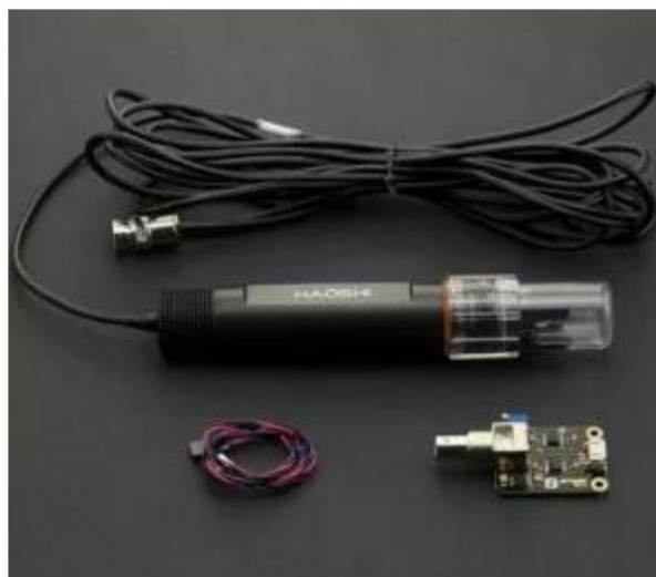
Figura 3.6: Sensor de pH industrial DFROBOT SEN0169.
